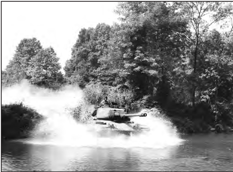
Figure 47. M41 light tank undergoing fording test.
