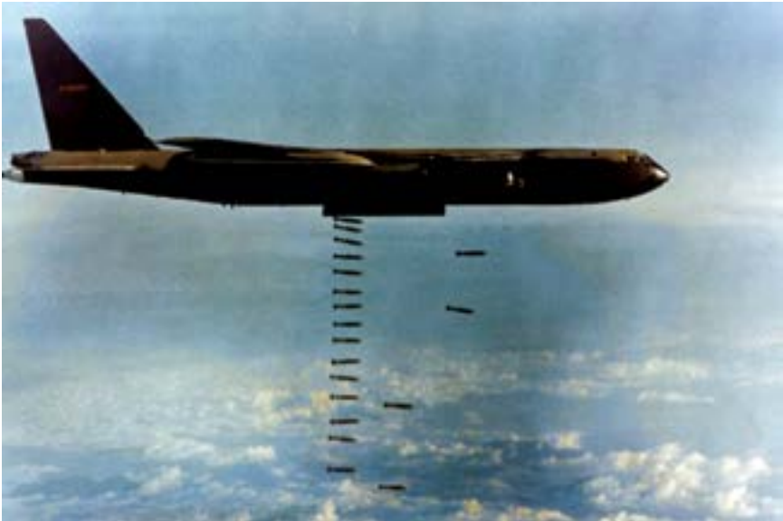
Figure 9.2 A US Air Force B-52D Stratofortress drops M117 750-pound bombs on a target in Southeast Asia. These eight engine bombers delivered punishing strikes during the 1970 Cambodia campaign. Photo courtesy of US Department of Defense.
