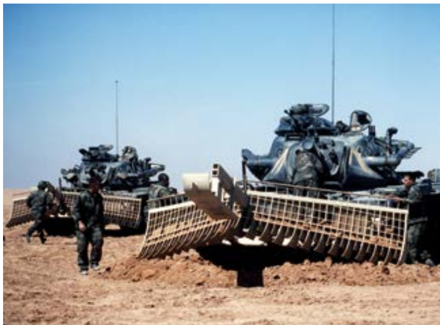
Figure 10.3. Members of the 72nd Engineering Company, 24th Infantry Division, test a mine-clearing rake attached to an M-728 Combat Engineer Vehicle. Photo courtesy of US Army Engineer School History Office.
