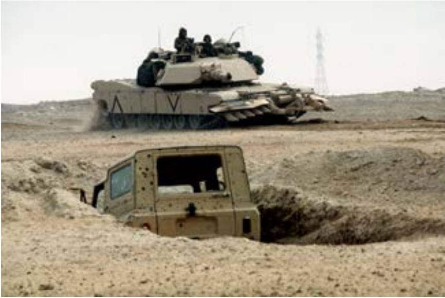
Figure 10.2. A Marine Corps M1A1 Abrams main battle tank equipped with a mine-clearing plow passes a truck in an abandoned Iraqi position. Photo courtesy of US Army Engineer School History Office.
