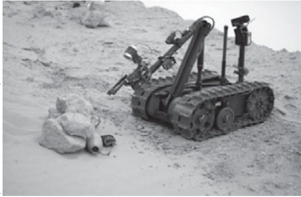
Robots such as TALON allow warfighters to clear routes quickly without having to wait for explosive ordnance disposal teams. Here a TALON robot inspects a suspected improvised explosive device.
