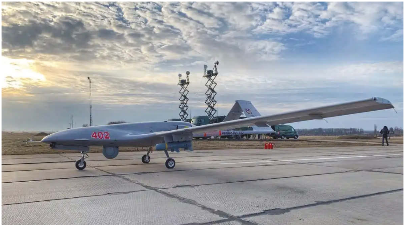
A Bayraktar TB2 drone of the Ukrainian Air Force armed with a MAM-L Smart Micro Munition guided bomb; two ground control stations are in the background. (Photo courtesy of Ministry of Defence of Ukraine via Wikimedia Commons)
