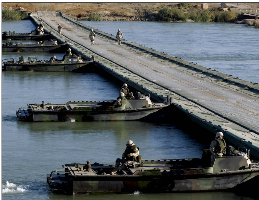
Figure 10.3. Bridge erection boats (BEBs) employed to stabilize an improved ribbon bridge (IRB) during training exercises. Courtesy of US Army.
