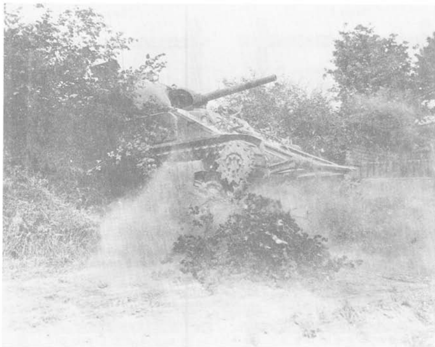
A Sherman tank crew practices using a hedgerow-cutter device prior to a battle
