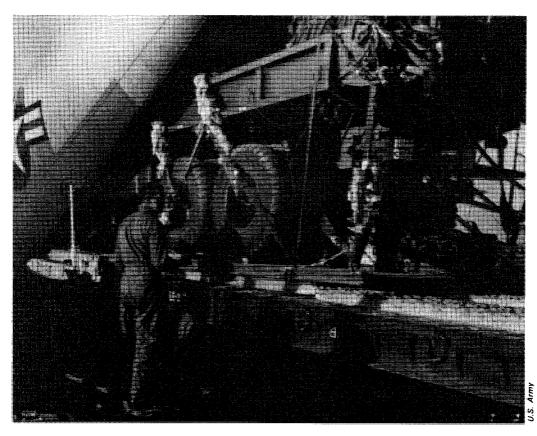
A 21/2-ton truck being rigged and loaded for airdrop aboard a C-130 transport
