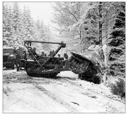
Figure 6.5. A bulldozer from the 307th Engineer Combat Battalion pushes a destroyed German armored vehicle off the snow-covered road during the Battle of the Bulge in early January 1945. This mobility function supported the American counterattack that drove the Germans back to the original front lines. Courtesy of US Army Engineer School History Office Archives.
