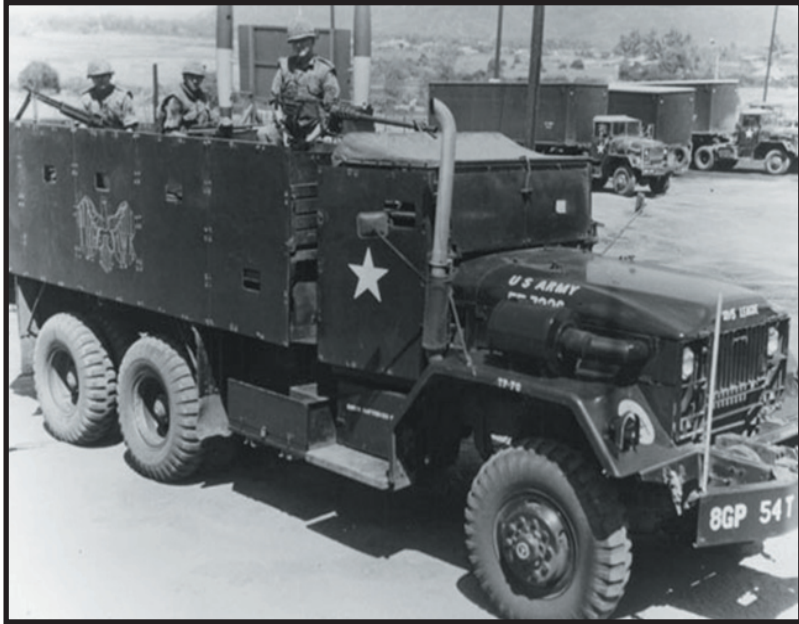
Figure 9. Gun Truck with Gun Ports and Windshield Cover.
