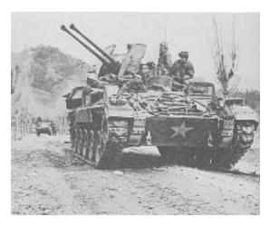
The M19 Multiple Gun Motor Carriage (MGMC) was originally developed as self-propelled anti-aircraft weapon on the M24 light tank chassis. It was equipped with two Bofors 40mmm guns mounted in a revolving turret. (4 in the 23<sup>rd</sup> RCT's B Battery, 503 AAA AW (SP) Battalion).
