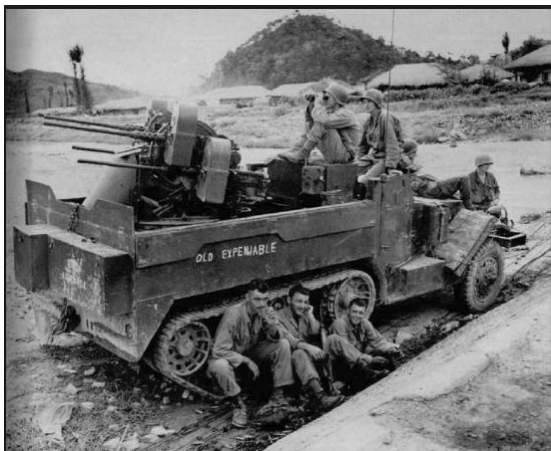
M16 MGMC - Quad .50: A half-track mounting four 50 cal. HMGs. It was originally developed as an anti-aircraft weapon in WWII. In Korea, it was primarily used as an antipersonnel weapon. It was capable of hurling an immense amount of fire onto hillsides against infantry. US soldiers referred to them as a “vacuum cleaner” or “ridge sweeper” that was capable of sucking the ridge until it was devoid of life. (8 in the 23 rd RCT’s B Battery, 503 AAA AW (SP) Battalion).
