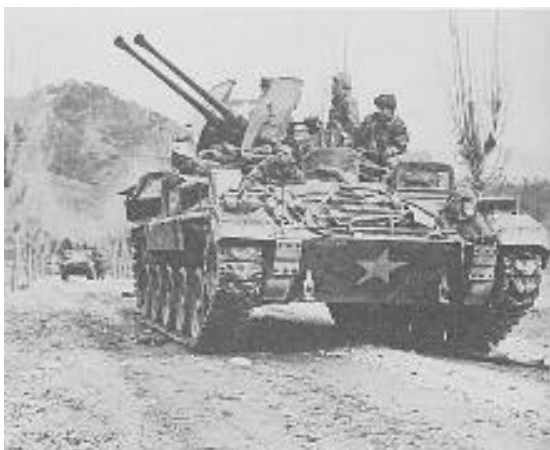
The M19 Multiple Gun Motor Carriage (MGMC) was originally developed as self-propelled anti-aircraft weapon on the M24 light tank chassis. It was equipped with two Bofors 40mm guns mounted in a revolving turret. (4 in the 23 rd RCT’s B Battery, 503 AAA AW (SP) Battalion).
