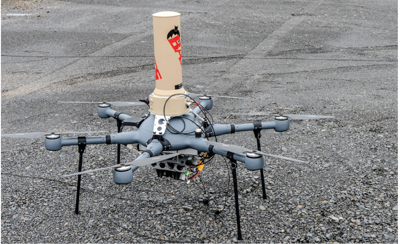
Industry partners combine a tethered drone, a directional antenna, and a radio to achieve a communications solution (HEMS VIIB) to digitally communicate a distance of eighty-seven miles from Fort Drum to the top of Whiteface Mountain (highest peak in New York State) on 5–8 December 2023. (Photo by Chief Warrant Officer 2 Michael [Brett] Melnyk, U.S. Army)
