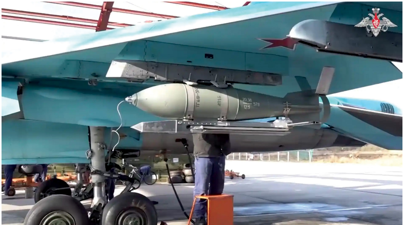
A 500 kg-class FAB-500 M-62 high-explosive bomb equipped with a UMPK guided glide kit is attached to the midboard port wing station of a VKS Su-34 strike fighter assigned to the 47th Bomber Aviation Regiment at Voronezh-Baltmor air base in Russia. (Still image courtesy of the Russian Ministry of Defence)
