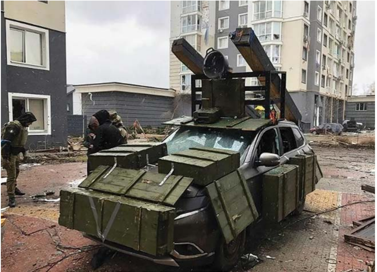
A passenger car is disguised as a Strela-10 anti-aircraft missile launcher May 2022 in Ukraine. Ukraine uses wooden decoys like this that resemble advanced rocket systems to trick Russian forces into attacking them using long-range cruise missiles. Reportedly, Russian drone sensors have had great difficulty in distinguishing Ukrainian decoys from actual rocket systems. (Photo courtesy of Novynarnia)
