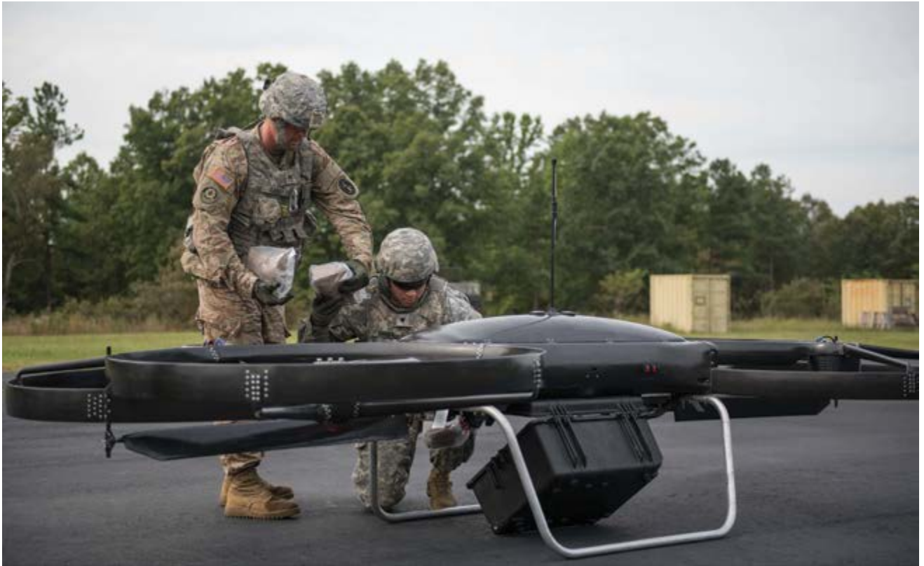
Soldiers of the 3rd U.S. Infantry Regiment participate in a Joint Tactical Aerial Resupply Vehicle (JTARV) exercise on Fort A. P. Hill, Virginia, 22 September 2017. During the exercise, the JTARV demonstrated its potential for soldiers on the battlefield to execute autonomous resupply. However, the JTARV is significantly restricted by range, capacity, and signature. (Photo by Pvt. Gabriel Silva, U.S. Army)
