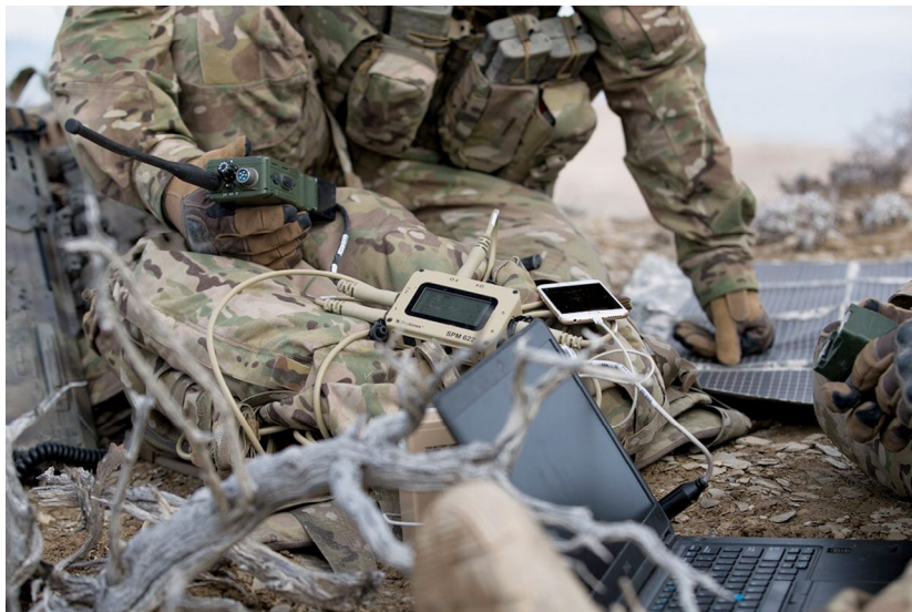
The SPM-622 Squad Power Manager will reduce power limitations and the battery weight carried by dismounted soldiers by enabling military forces to manage and prioritize power use for various electronics devices—including portable radios, GPS systems, medical and explosive ordnance disposal equipment, and computers—from any available power source. (Photo courtesy of Revision Military)
