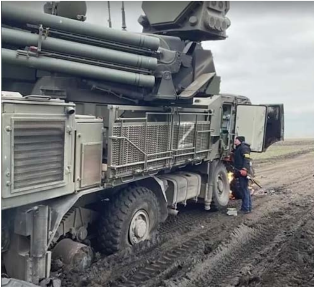
A disabled Pacir-S air defense vehicle sits mired in the mud in Ukraine. Disintegrated tires on Russian combat vehicles and trucks in Ukraine are a sign of poor basic maintenance. (Screenshot courtesy of Crux via Youtube)
