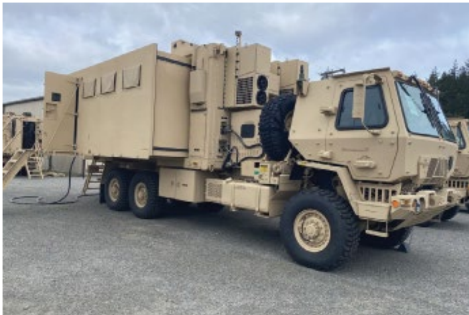
An M1087 Expandable Van Shelter houses the Command Post Integrated Infrastructure System under operational test by the 2nd Infantry Division's 2nd Stryker Brigade Combat Team at Joint Base Lewis-McChord, Washington. (Photo by Sgt. 1st Class Frederick E. Estep, U.S. Army Operational Test Command)
