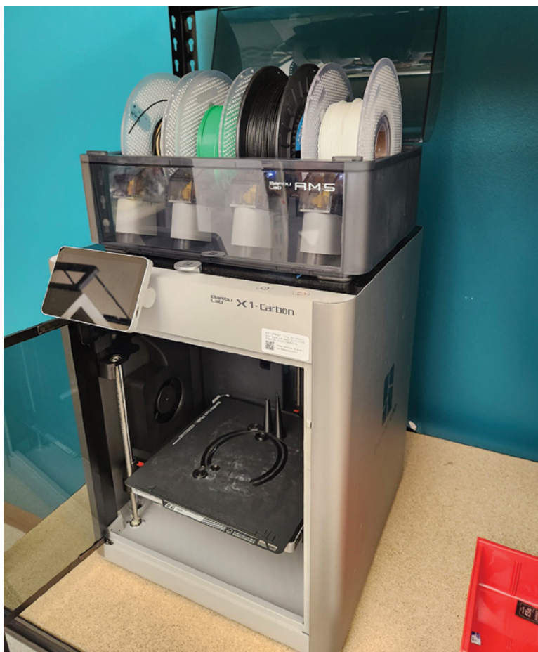
A benchtop fused deposition printer. The spools of black, green, and white filament are visible in the top storage compartment. This printer melts, or fuses, the spools together to produce items. (Photo by Lt. Col. Andres Mendoza, U.S. Army Institute of Surgical Research)
