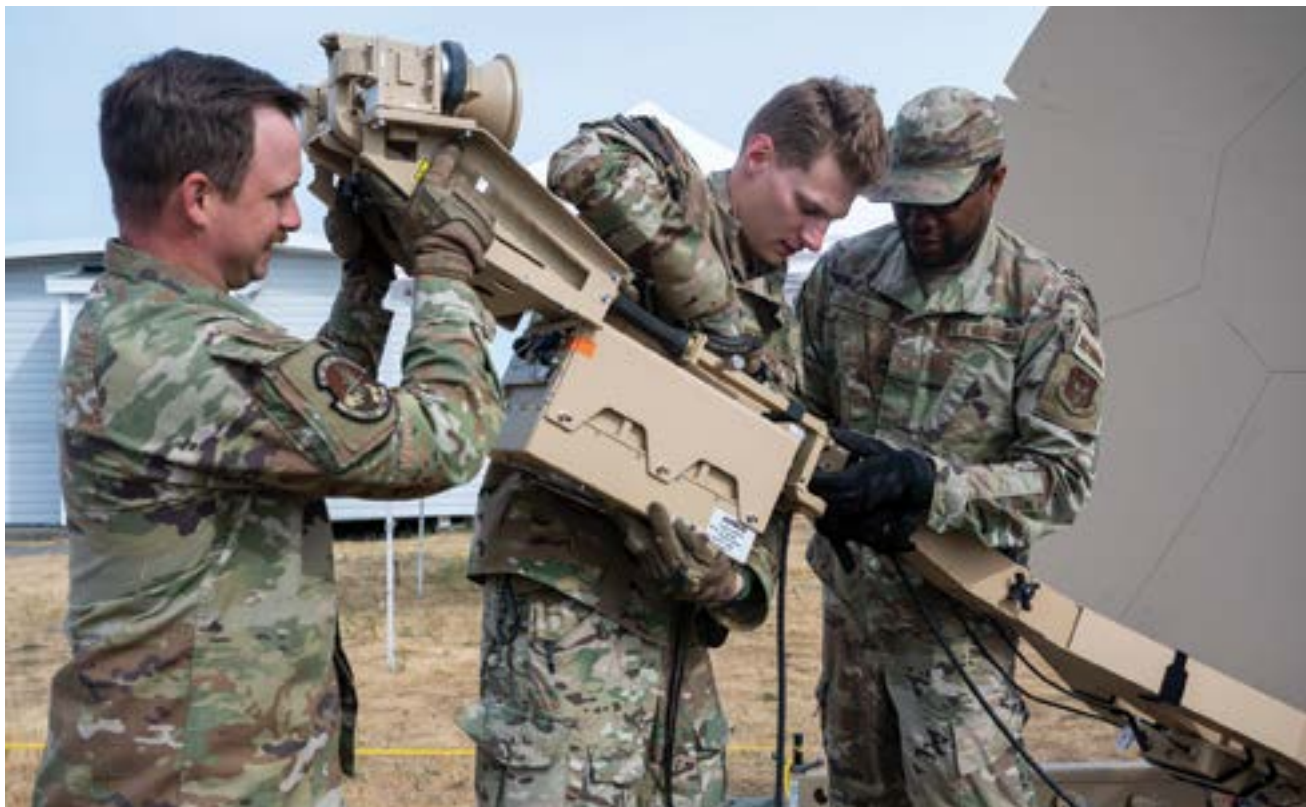
Airmen with the 35th and 55th Combat Communications Squadrons replace a feed boom on a Ranger 2400 Flyaway Multi-Band Terminal during Exercise Agile Blizzard-Unified Vision 2023 near Comox, British Columbia, Canada, 19 June 2023. The satellite dish allows for quick setup satellite communications that are necessary when operating in a semi-austere location where communications are limited. (Photo by Tech. Sgt. Betty R. Chevalier, U.S. Air Force)
