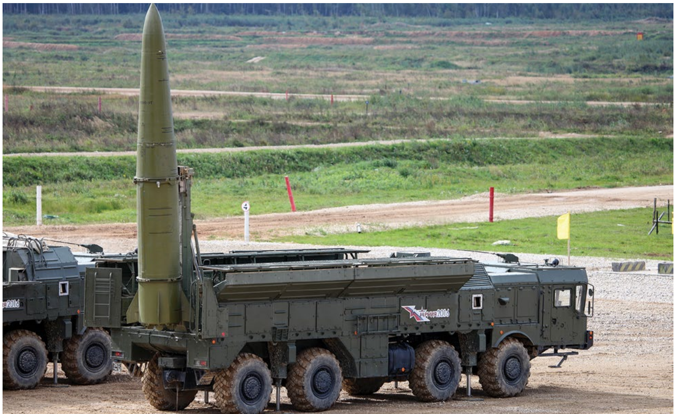
A self-propelled launcher 9P78-1 OTRK 9K720 Iskander-M with a 9M723K5 missile. The short-range ballistic missiles can reach hypersonic speeds of 2,100 to 2,600 meters per second. (Photo by Vitaly Kuzmin via Wikimedia Commons)
