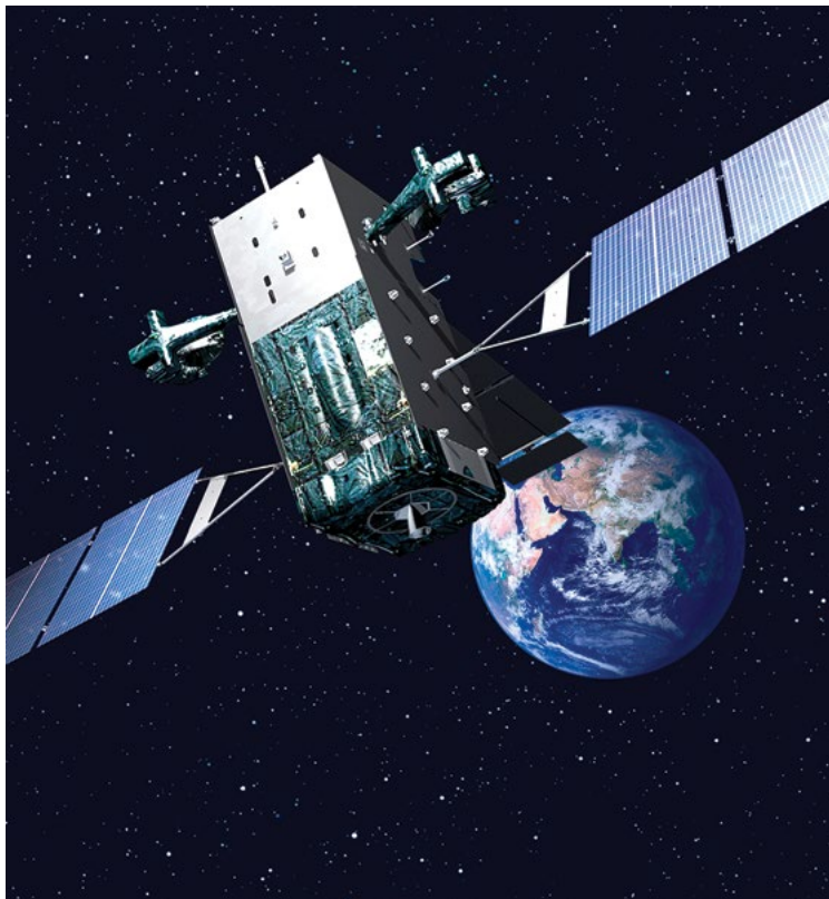
A depiction of a Space-Based Infrared System (SBIRS) satellite. The SBIRS is designed to support missile early warning, missile defense, and intelligence collection. (Image courtesy of the U.S. Space Force)
