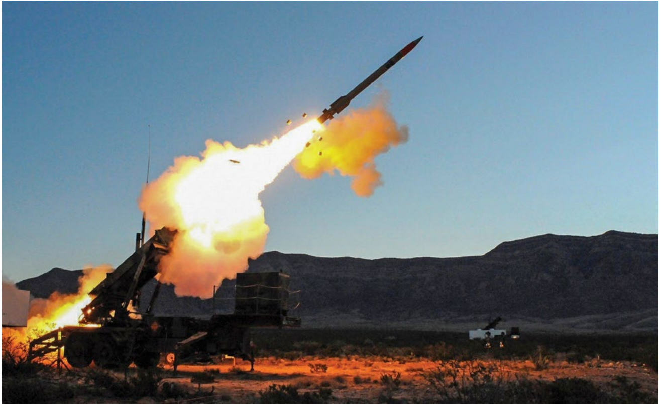
The U.S. Army fires a Patriot missile in a 31 March 2019 test. The Patriot missile system is a ground-based, mobile missile defense interceptor deployed by the United States to detect, track, and engage unmanned aerial vehicles, cruise missiles, and short-range and tactical ballistic missiles. (Photo courtesy of U.S. Army Security Command)
