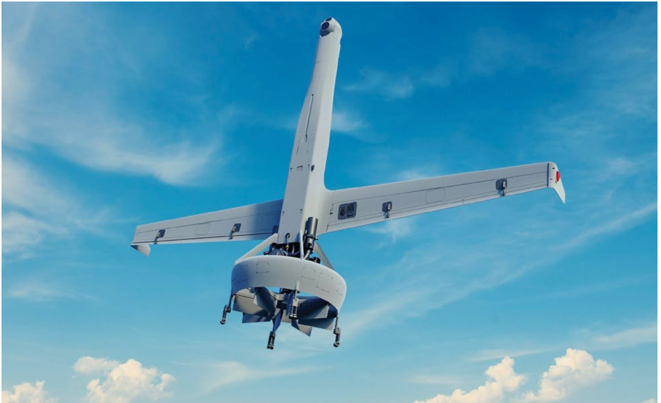
The Northrup Grumman and Shield AI V-BAT is one of five project agreement holders for the Future Tactical Unmanned Aircraft System (FTUAS) Increment 2 rapid prototyping effort. The FTUAS is the Army's premier vertical take off and landing unmanned aircraft modernization effort. Shield AI and Sentient modified the V-BAT with AI imagery to detect and classify machine-invisible targets on the move. (Photo courtesy of Shield AI)
