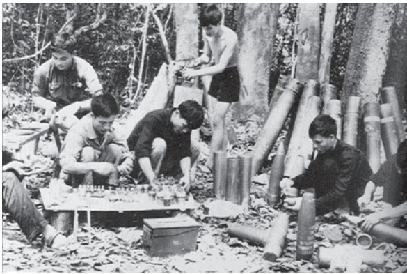
Vietcong remanufacturing satchel charges and other explosives by cannibalizing captured allied artillery shells.
