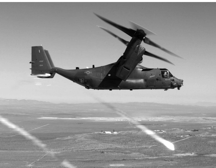
The CV-22 Osprey fires countermeasures during a safe-separation test over the precision impact range area at Edwards Air Force Base, California, in 2004.
