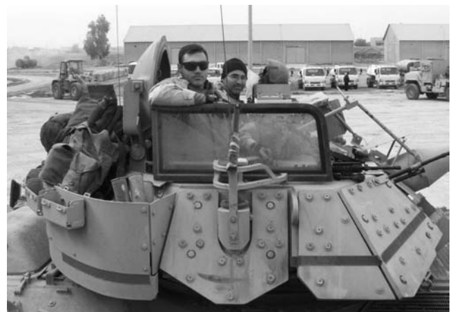
A 2d Squadron Bradley modified with up-armored windshields to protect Bradley commanders from IEDs, February 2006.
