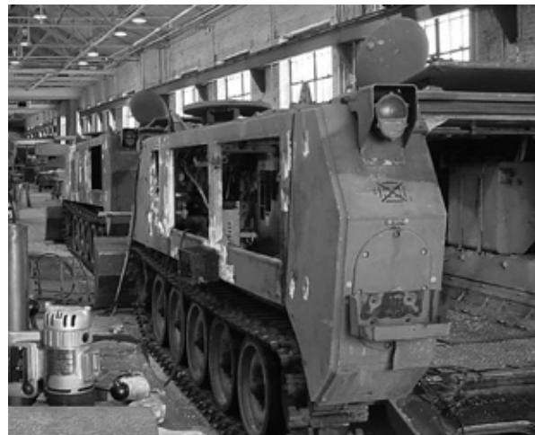
Rapid entry vehicles (REVs) on the assembly line at Picatinny Arsenal, New Jersey, 2006. The REV is a modified M113 armored personnel carrier used for nonlethal crowd control and rescue squad insertions. The modifications include cutting large holes in the hull and installing ballistic glass windows and Bradley firing ports, which increase Soldier survivability through improved situational awareness and mobility.
