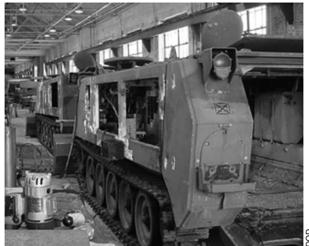
Rapid entry vehicles (REV)s on the assembly line at Picatinny Arsenal, New Jersey, 2006. The REV is a modified M113 armored personnel carrier used for nonlethal crowd control and rescue squad insertions. The modifications include cutting large holes in the hull and installing ballistic glass windows and Bradley firing ports, which increase Soldier survivability through improved situational awareness and mobility.
