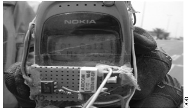
This cell phone was rigged as a detonator for an improvised explosive device. The detonator was recovered undamaged after having been successfully jammed by electronic warfare personnel using Counter Radio-Controlled IED Electronic Warfare equipment funded by the Joint IED Defeat Organization.
