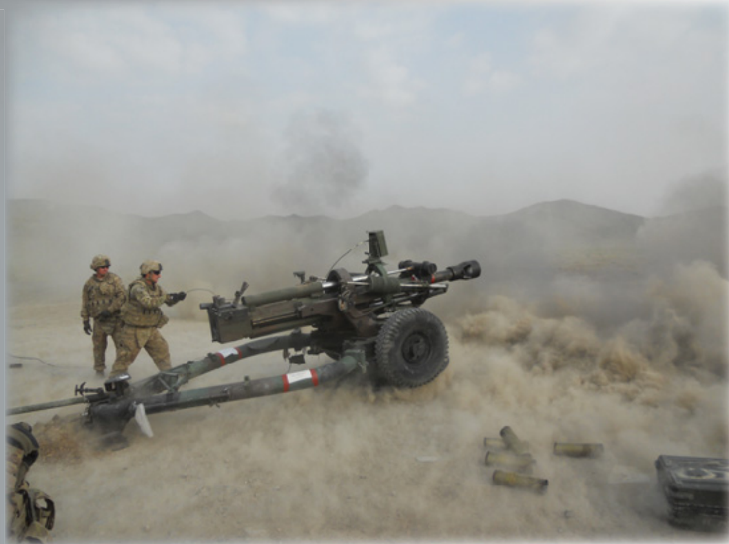
Cannoneers from Battery A, 1st Battalion, 6th Field Artillery Regiment, Task Force Centaur, fire maximum charge 8 from their M119A2 howitzer in support of operations in Khost Province, Afghanistan, 21 July 2011. (U.S. Army, LTC James W. Vizzard).
