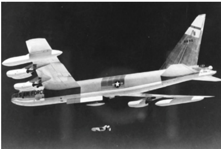
A B-52D shown conducting a launch of an ADM 20 Quail decoy. (U.S. Air Force)
