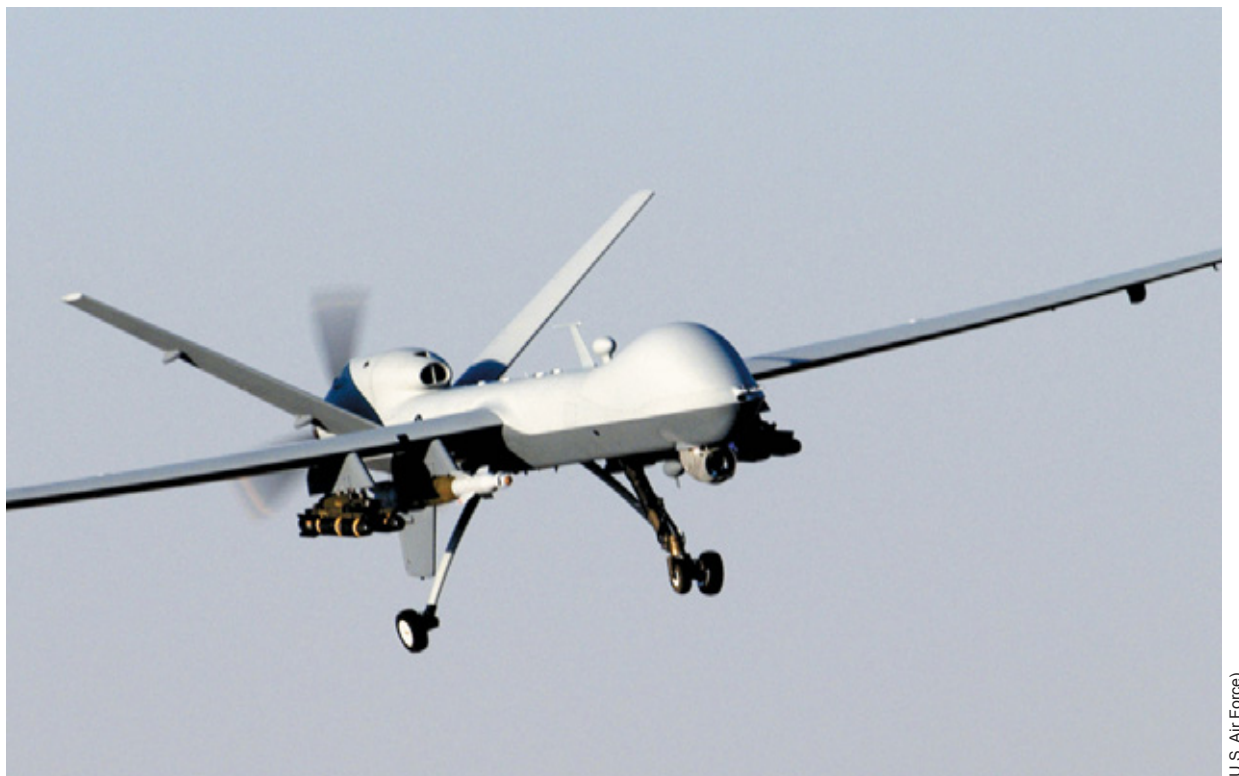
An MQ-9 Reaper unmanned aerial vehicle prepares to land after a mission in support of Operation Enduring Freedom in Afghanistan, 17 December 2007. The Reaper has the ability to carry both precision-guided bombs and air-to-ground missiles.
