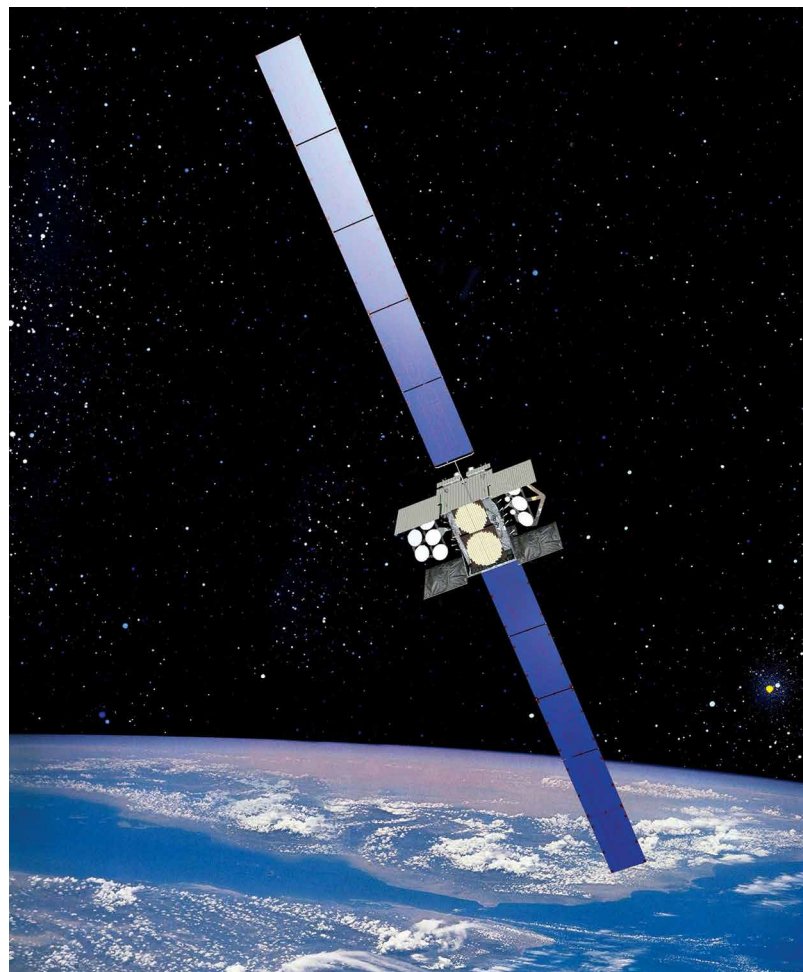
A Wideband Global SATCOM satellite has the constructive effect of providing roughly twelve times the bandwidth of previous systems. (Photo courtesy of Boeing)
