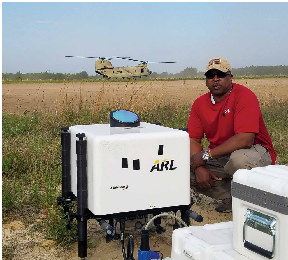
Deryck James, Army Research Laboratory (ARL), operates the Stream Line PRO Light Detection and Ranging (LiDAR) at the Parachute Operations Mishap Prevention Orientation Course 2016, Fort Stewart, Georgia, to demonstrate enhanced capabilities not available with current precision airdrop operations systems. In response to a request from United States Army Africa, ARL undertook a program to reduce the size, weight, and power of current commercial off-the-shelf Doppler LiDAR systems. The new system weighs less than forty-five pounds, is under two cubic feet, and operates on standard twenty-four-volt batteries with required power of less than one hundred watts. (Photo courtesy of U.S. Army)
