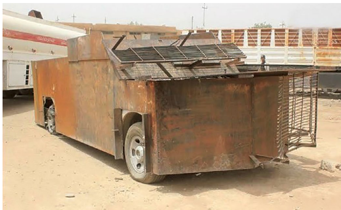
The Islamic State uses trucks such as the one shown above, captured near Kirkuk, Iraq, in 2015, as vehicle-borne improvised explosive devices driven by suicide bombers. The vehicles are fitted with improvised armor to protect the trucks and their drivers until detonation. Note the grills intended to defeat rocket-propelled grenades. (Photo courtesy of Ministry of Peshmerga Affairs)
