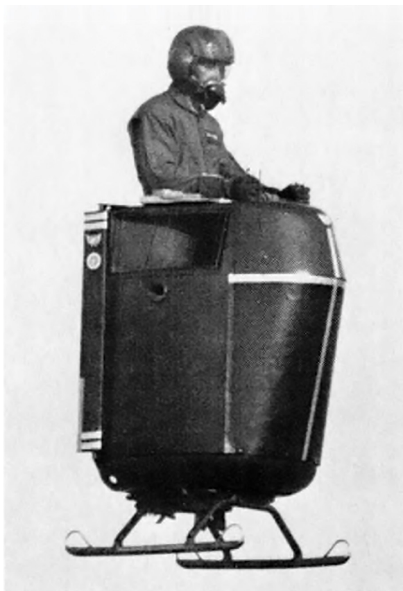
A turbine-powered individual lift device designed to take off vertically and enable a man to fly for thirty minutes at speeds of up to sixty miles per hour has been successfully flown in a series of free flights by military personnel. It is known as the Williams Aerial Systems Platform (WASP II). The WASP II was considered as a candidate individual lift device by the Army and the Infantry Board in the 1980s. (Photo courtesy of the U.S. Army)
