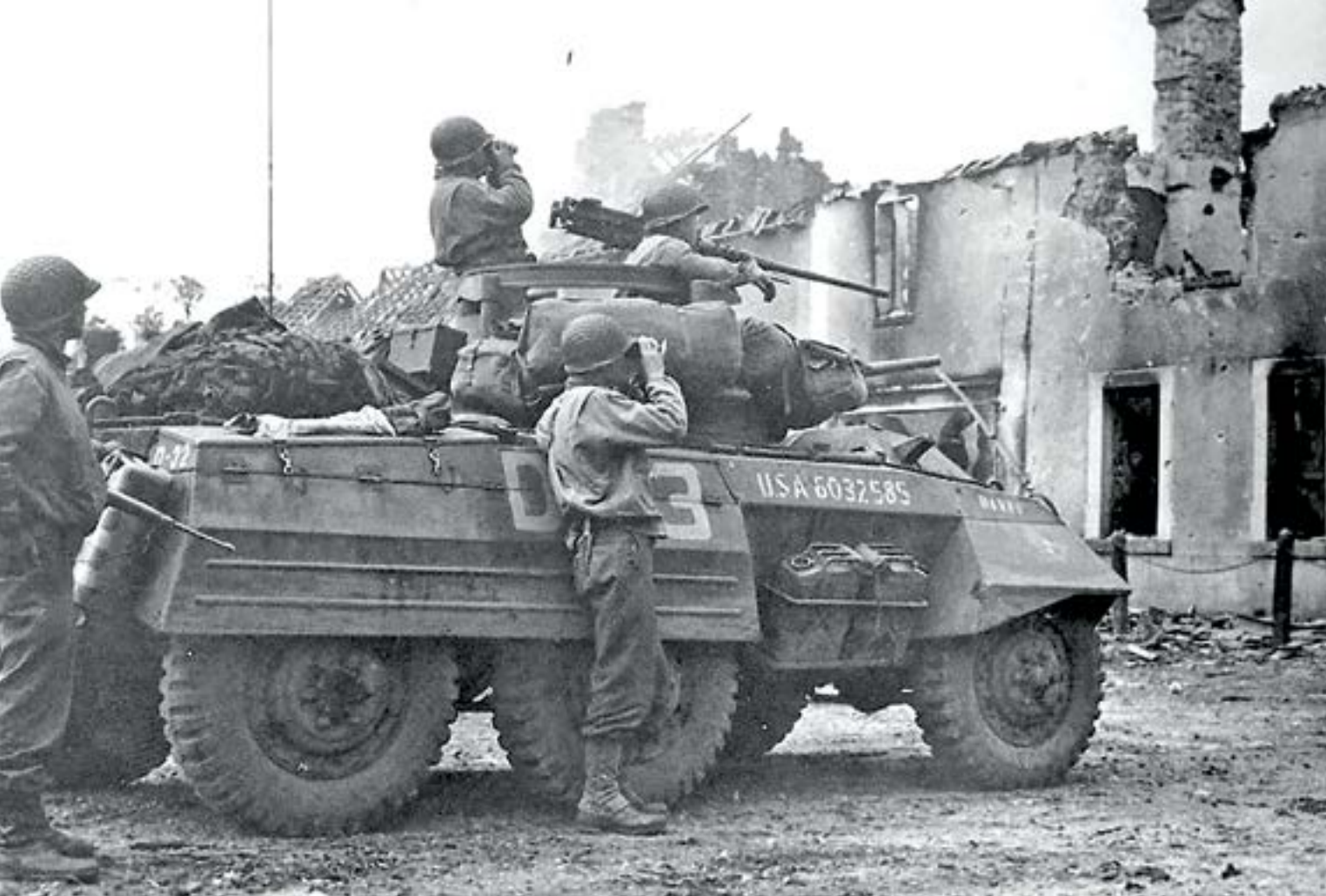
An M8 Light Armored Car is used to conduct reconnaissance during World War II circa 1944. The M8, sometimes referred to as the Greyhound, was provided to cavalry units as a reconnaissance vehicle. It could travel at speeds of 55 mph and had excellent on-road mobility, which made it especially useful for operations on the well-developed road systems of Europe. It was equipped with a long-range radio and was armed with a 37 mm gun and either a .30-caliber or .50-caliber machine gun. The M8 proved very versatile and was widely used by cavalry units for reconnaissance and to support screening missions both during World War II and for decades after the war. (Photo courtesy of War History Online, www.warhistoryonline.com )
