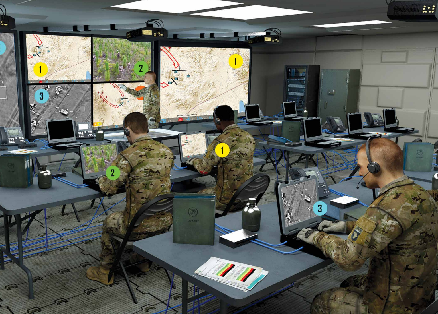
The digital viewer application, or DVA, provides the Army with a software-based video switching solution and allows command post personnel to connect to the local area network to share all or part of their display with other individuals or on the larger command post display system. (Photo simulation courtesy of the U.S. Army)
