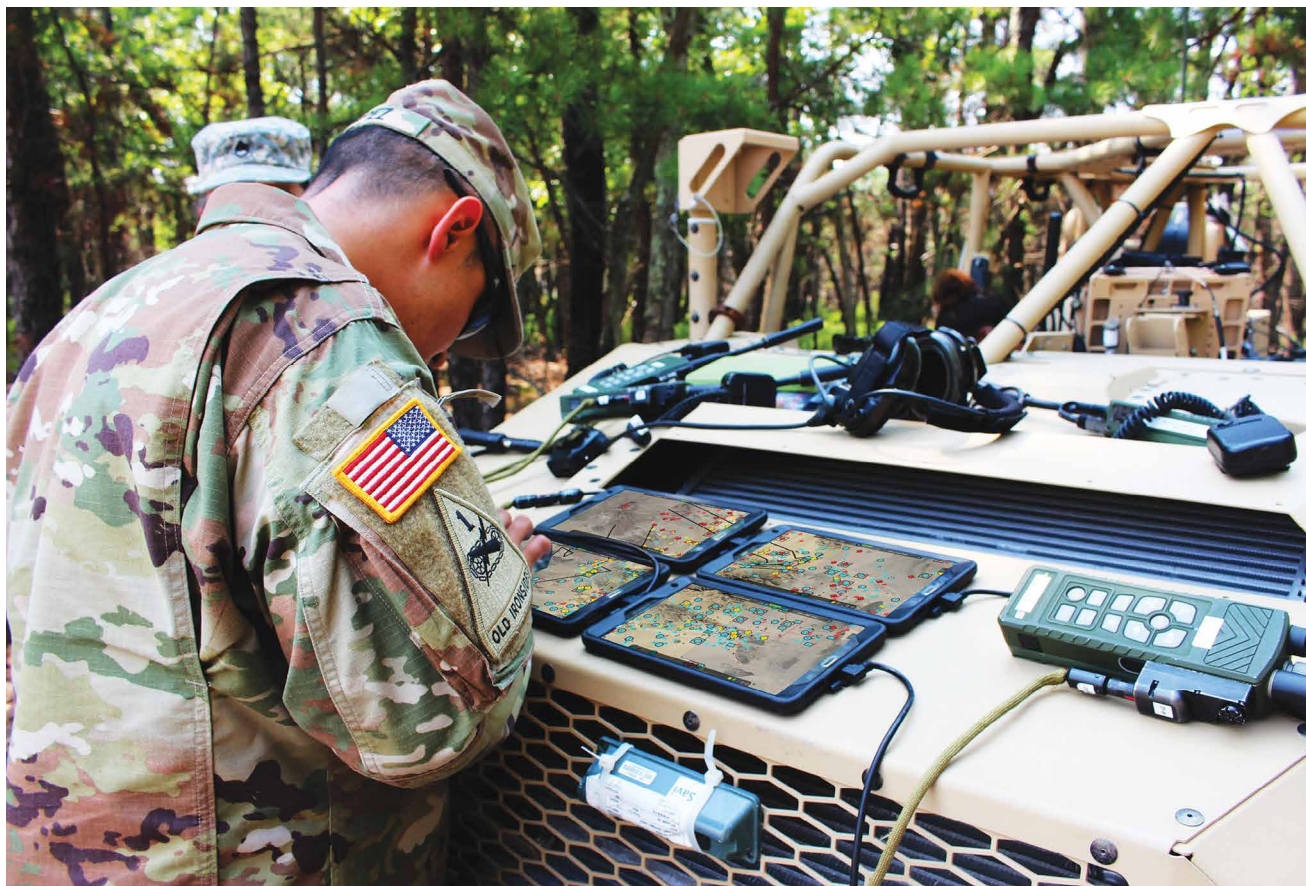
Soldiers configure the tactical computing environment extend mode, which pieces together various points on a digital map to create one, large map-view similar to what is available in larger command posts. This technology can help soldiers collaborate and increases situational awareness across a formation by sharing a near real-time common operating picture of the "data-swept battlefield." (Photo courtesy of the U.S. Army)
