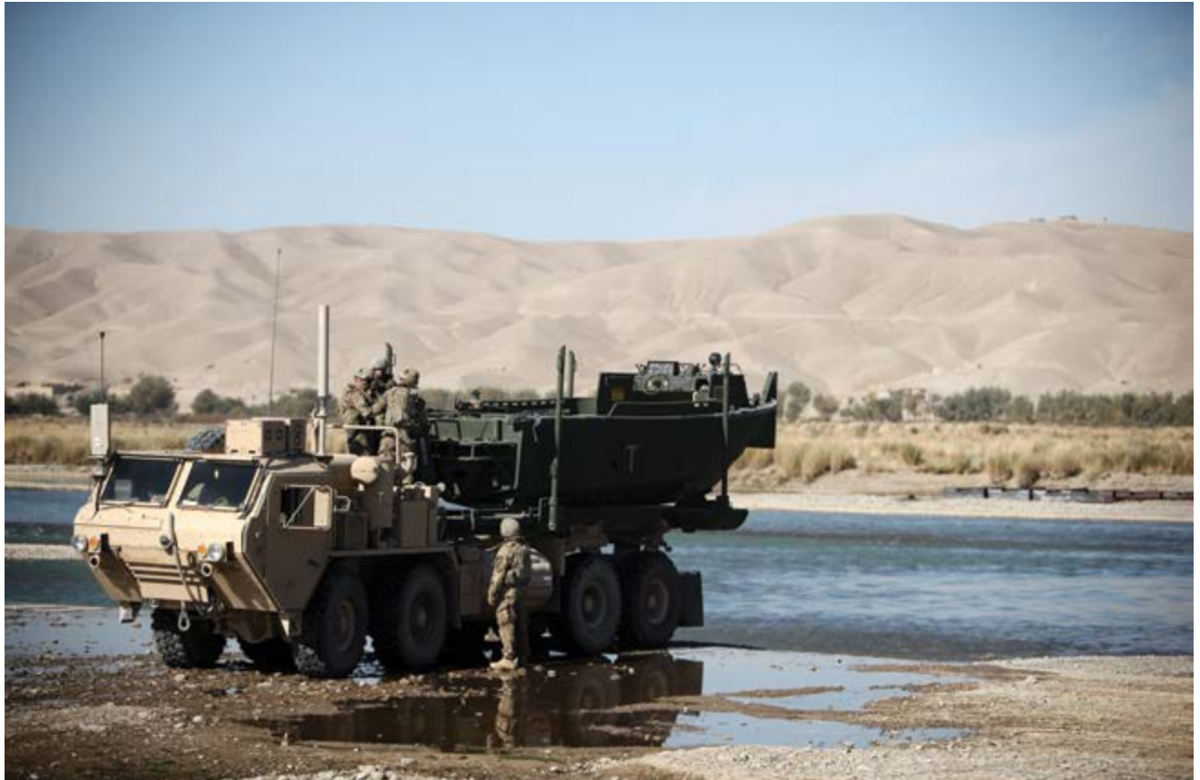
Army engineers from the 132nd Multi-Role Bridge Company prepare a bridge erection boat for employment on 7 November 2012 outside of Forward Operating Base Jackson in Helmand Province, Afghanistan. The 132nd “River Rats” provided construction and bridge repair support for Operation Golden Gate, a bridge-building operation allowing the Afghan population to cross the Helmand River safely from the Musa Qal’ah District into the Sangin District. Infrastructure improvement was one of the tools used by U.S. forces in their efforts at nation building. (Photo by Lance Cpl. Alexander Quiles, U.S. Marine Corps)
