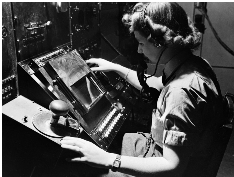
Women's Auxiliary Air Force radar operator Denise Miley plots aircraft on the cathode ray tube of an RF7 receiver in the Receiver Room at Bawdsey Chain Home (CH) in England, circa 1945. Her right hand has selected the direction or height finding and her left hand is ready to register the goniometer setting to the calculator. RAF Bawdsey was originally an experimental system set up at Bawdsey Manor, home of Robert Watson-Watt's radar development team. When the team was moved away from Bawdsey, the radar station became a part of the operational CH network. (Photo courtesy of the Imperial War Museums)
