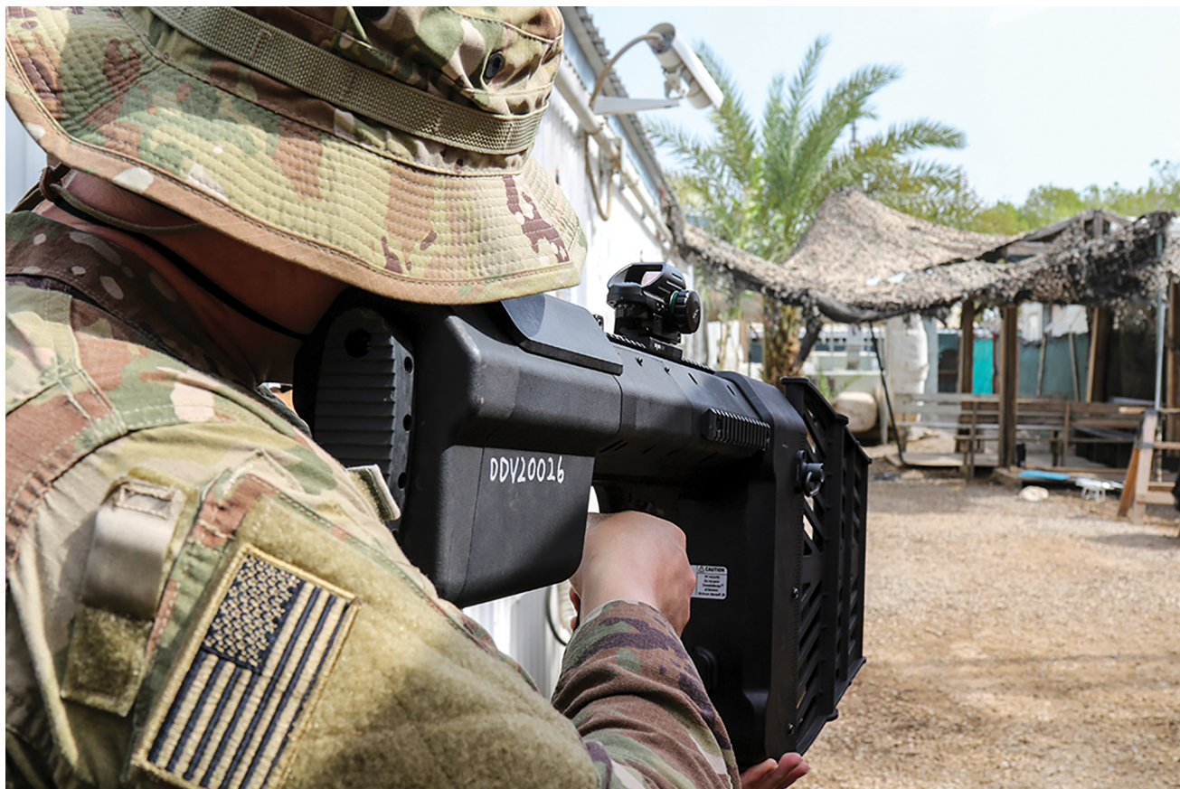
A soldier with Company B, 2nd Battalion, 135th Infantry Regiment, looks through the optic device of the Drone Defender V2 during counter unmanned aircraft systems training at Camp Lemonnier, Djibouti, 19 August 2020. The Drone Defender V2 is an electronic warfare weapon that is capable of downing and disabling a small unmanned aircraft system. (Photo by Sgt. Sirrina Martinez, U.S. Army)
