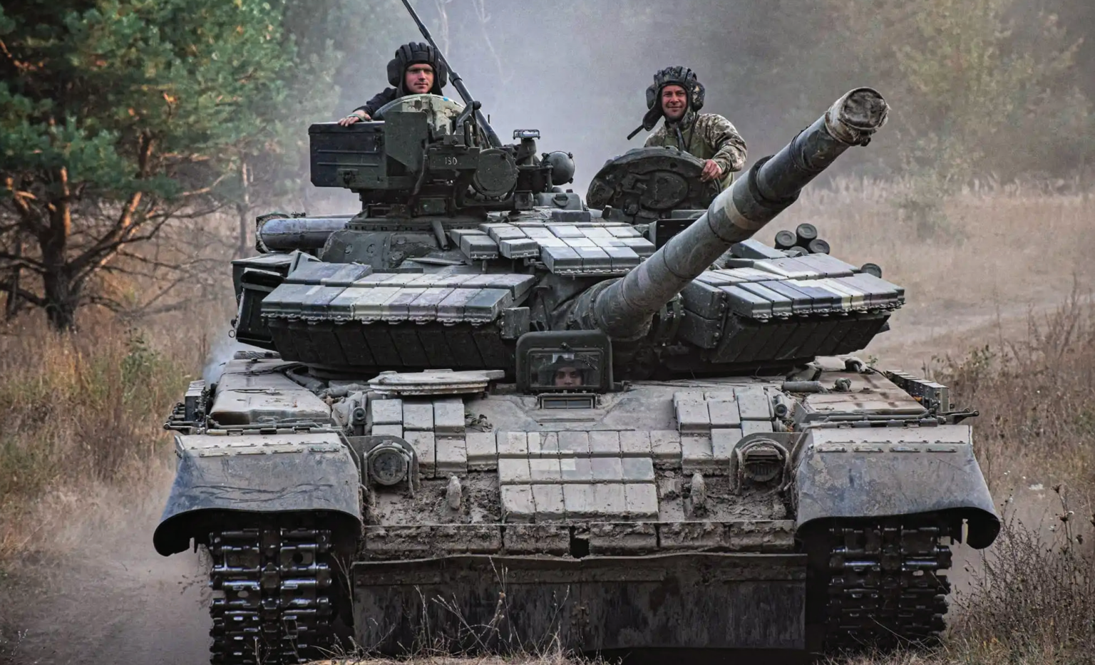
A Ukrainian T-64 BV tank from the 59th Yakiv Handziuk Motorized Brigade maneuvers in September 2022. Originally designed in the Soviet Union during the 1960s, it benefited from upgrades over the years, including Ukrainian improvements to its thermal imaging, reactive armor, and radio. (Photo courtesy of the Ministry of Defense of Ukraine via Wikimedia Commons)
