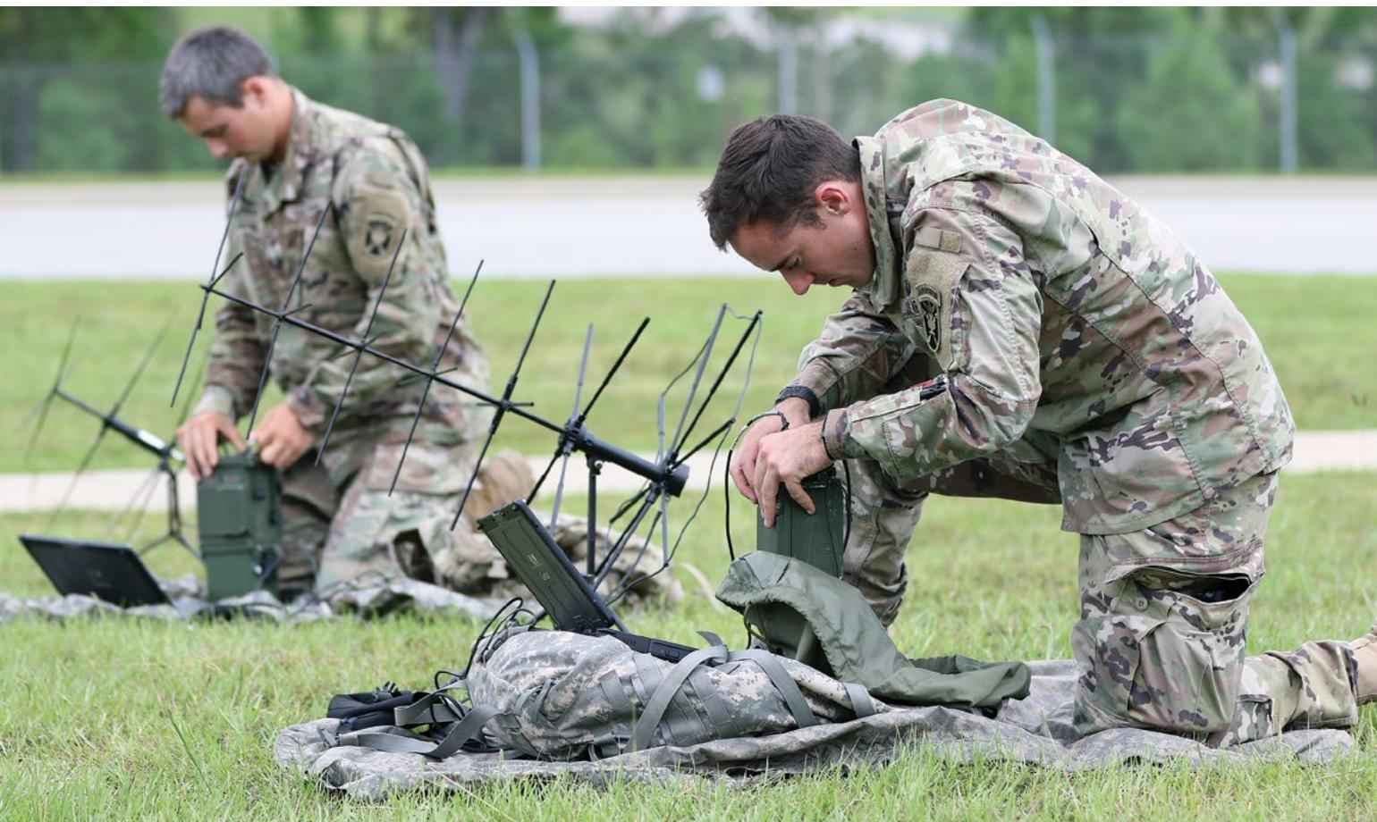
Soldiers in the Special Forces Communications Sergeant Course practice using a PDA-184 computer and an AN/PRC-117G satellite radio 29 August 2019 at the Yarbrough Training Complex, Fort Bragg, North Carolina. The satellite communications module qualified students to be proficient in installing, operating, and maintaining a satellite communications link. (Photo by K. Kassens, U.S. Army)
