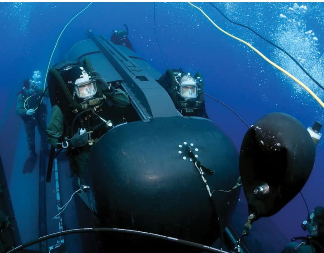
U.S. Navy SEAL Delivery Vehicle Team 2 launches a SEAL Delivery Vehicle (mini submarine) from the Los Angeles-class submarine USS *Philadelphia*. Such teams provide a specialized capability for conducting covert infiltration and exfiltration littoral operations in regions of potential conflict such as the South China Sea. (Photo by Chief Photographer's Mate Andrew McKaskle, U.S. Navy)
