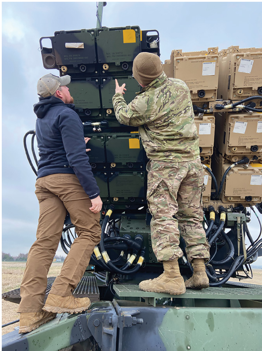
Kyle Battles, a U.S. Army Joint Munitions Command quality assurance specialist (ammunition surveillance), checks the humidity indicator on a Patriot surface-to-air missile system in Żagań, Poland, 18 April 2022. (Photo courtesy of the U.S. Army)
