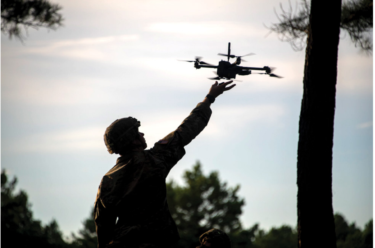
A 199th Infantry Brigade Experimental Force soldier hand-launches the Rucksack Portable Unmanned Aircraft Systems (RPUAS) on 19 August 2020 at Fort Moore, Georgia, during a named area of interest reconnaissance mission. RPUAS is a short-range reconnaissance drone within a family of aerial systems that span short-, medium-, and long-range reconnaissance. (Photo by Tad Browning, U.S. Army Operational Test Command)
