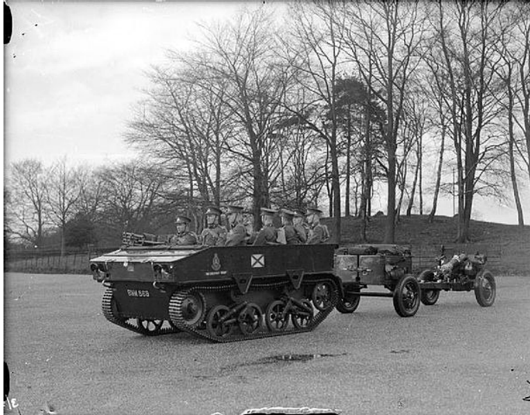
A Vickers Light Dragon field artillery tractor tows a limber (two-wheeled cart) and a 3.7 inch howitzer of A Battery (The Chestnut Troop), Royal Horse Artillery, British Army, in 1938. (Photo courtesy of Wikimedia Commons)
