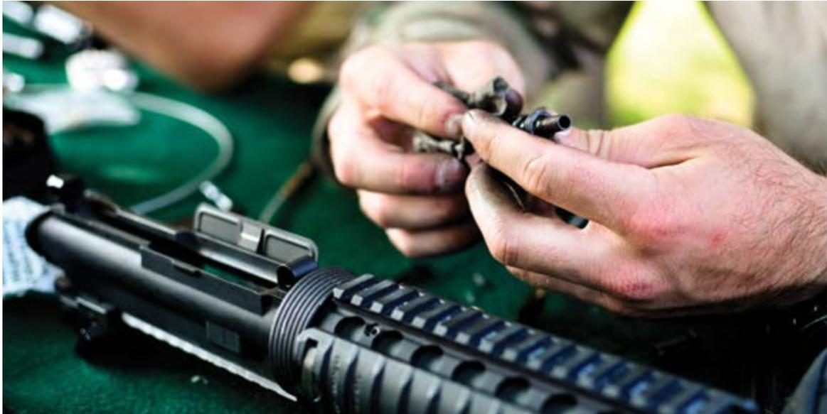
given an m4-series rifle, place the weapon on a clean flat work surface. ensure the weapon is on safe, remove any magazine,
