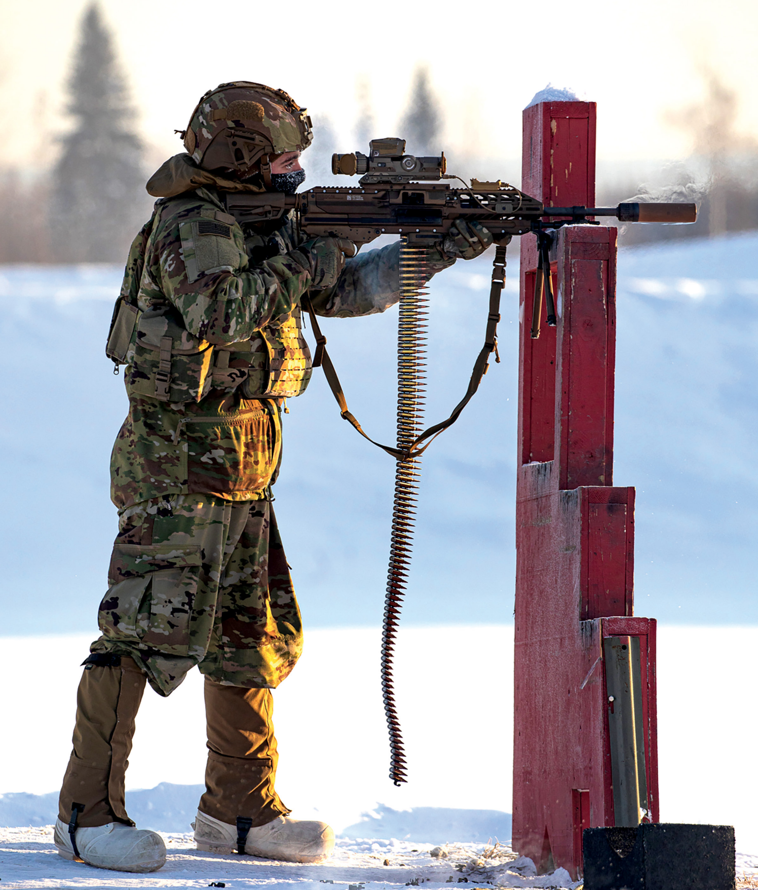
The U.S. Army Cold Regions Test Center tests the Army's Next Generation Squad Weapon at Fort Greely, Alaska, 23 January 2024. The XM7 and XM250 are successors to the M4 rifle and M249 light machine gun that U.S. forces have used for decades. The new weapons boast improved accuracy and range, weigh less, and fire with less recoil even though the 6.8 mm round is larger than the two legacy weapons' 5.56 mm cartridge. (Photo by Sebastian Saarloos, U.S. Army)
