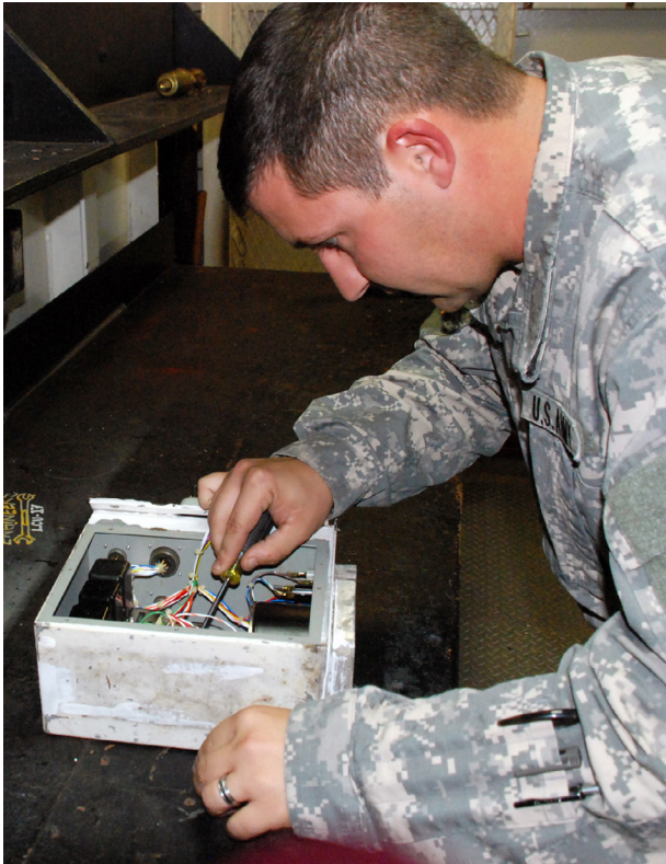
Sgt. Ryan Light, a junior marine engineer aboard one of 97th Transportation Company's Landing Craft Utility vessels, examines a tank level indicator, or TLI, that shows the amount of sewage being held on the vessel. "The TLI went out," Light said. "We pulled it apart and found that this transformer in here is blown." As part of their normal duties, engineers monitor the vessel's fuel, oil, sewage and drinking water. (Photo by Meghan Portillo)
