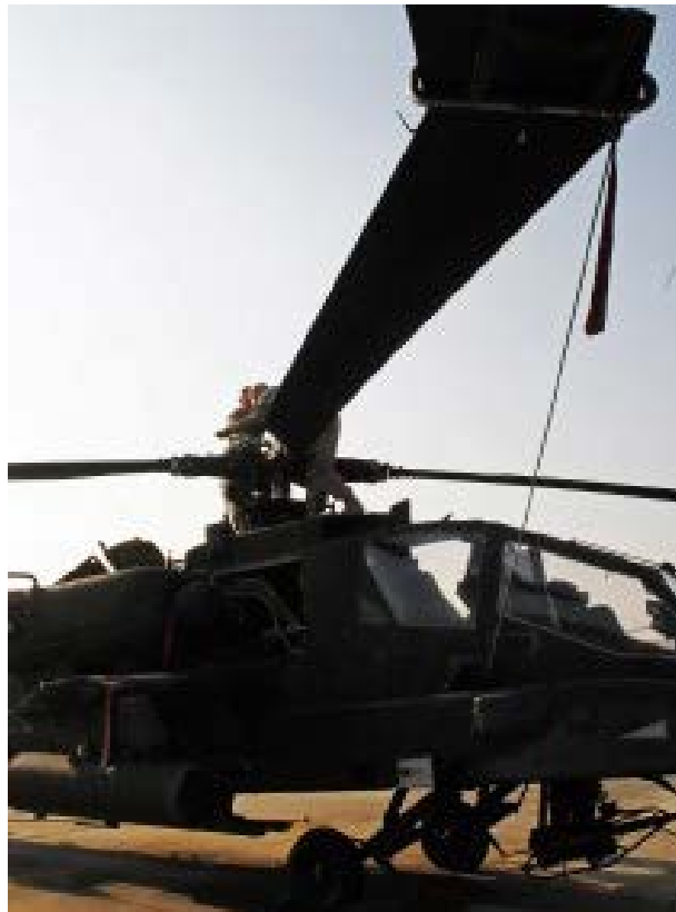
Sgt. David Henson and Spc. Justin Stack work on removing the pitch control links on a helicopter at Camp Humphreys, South Korea. Henson said NCOs in Korea get lots of experience teaching and mentoring young Soldiers. (Photos by Jonathan (Jay) Koester)
